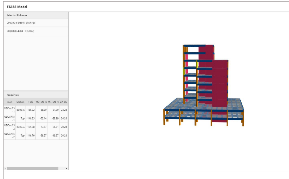
Figure 3.3 Importing Columns from ETABS Model
